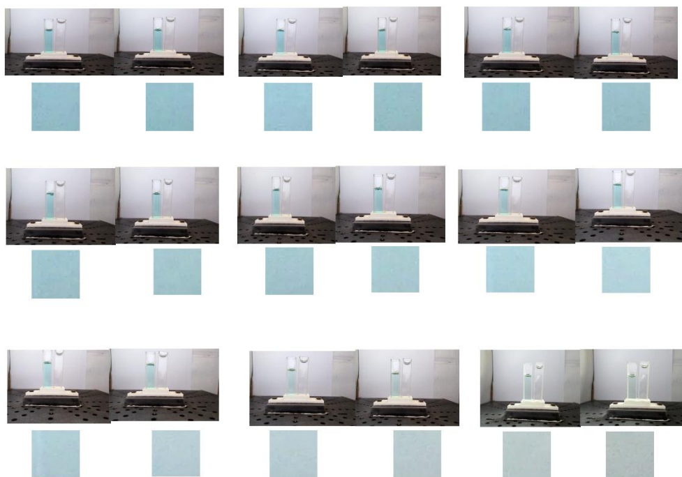
Fig. 2. Original Digital images and cropped images of MB- \text{HS}^- - \text{Se(IV)} cuvettes captured after 10 and 40 sec of pushing the start button and following the recommended procedure. From upper left to right, 0, 2, 4, 6, 8, 11, 14, 17, and 20 \text{ ng mL}^{-1} \text{Se(IV)} , respectively.
