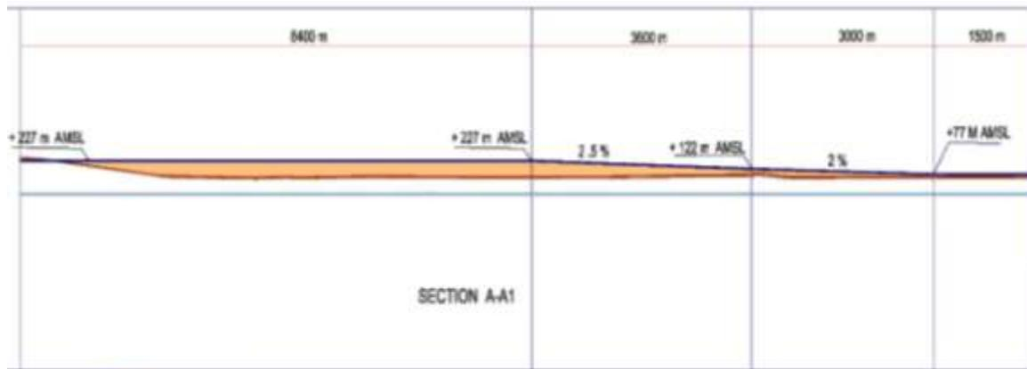
Fig. 11. (Section A-A) illustrates the relationship between Approach surface elevations and natural earth in longitudinal direction of runway (north - south direction).
